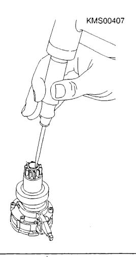
Disassembling overrunning-clutch drive
